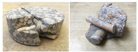
Fig. 5—GFRP coupons extracted from the concrete cores of Walker (left) and Southview (left) Bridge
